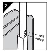
With ON/OFF switch facing the front of the unit, slide upper handle section over matching section of the connector assembly. Insert short screw into top hole and long screw into bottom hole then tighten firmly until handle is no longer loose.
